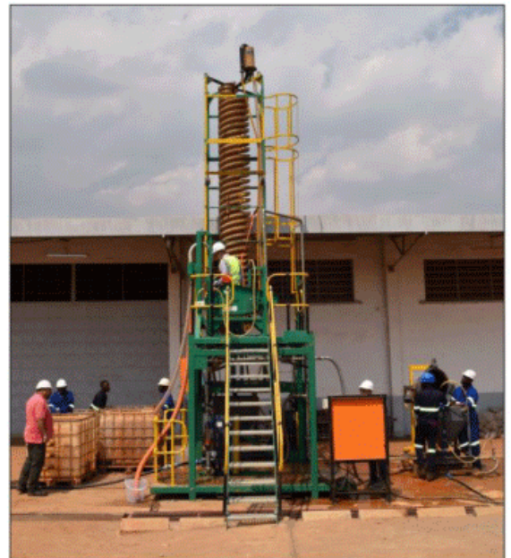
Figure 2: Commencement of spiral commissioning
