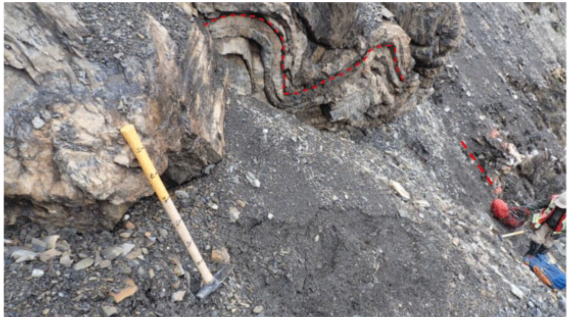
Chip Sample D – 723223 – 0.25 % copper over a width of 0.40 meters, elevation 1,902 meters Note strong folding.
