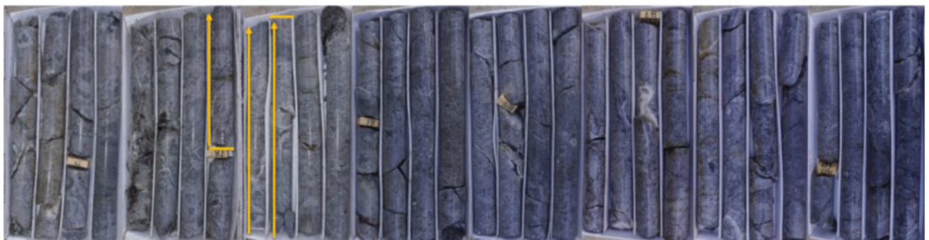
SM20- 43; 75m - 88.5m, 13.5m Polymictic Breccia. 78.00 m - 79.50 m, 1.50 meters grading 68.77 g/t Ag Eq
