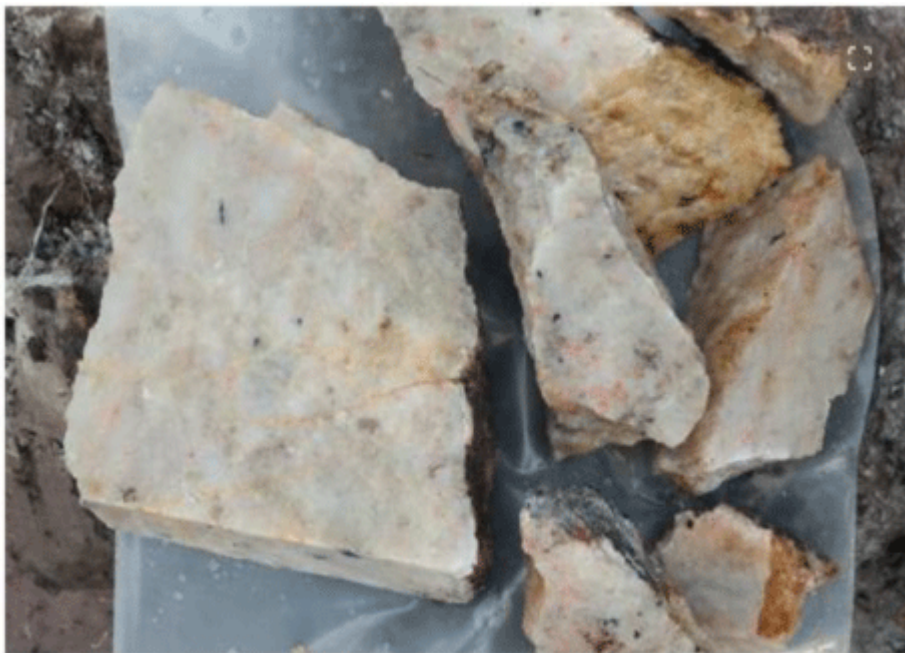
Figure 3: Channel sample at the newly discovered Cosma Caesium Pegmatite, assaying 0.5 m at 16.43% Cs 2 O.
