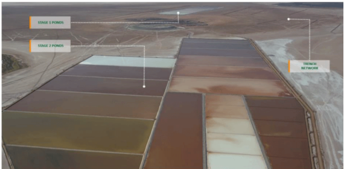
Figure 3: Stage 2 ponds, Stage 1 ponds & trench network
