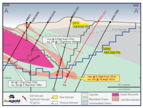
Figure 3 – Cross-section A-A' (6,288,080mN) across the Jinkas -White Dam Lodes with Resource
