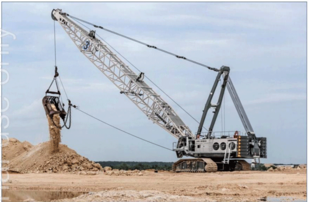
Figure 1: Example of a dragline excavator in action (Source: Liebherr)
