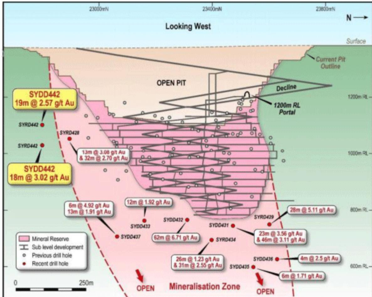
Figure 1: Longitudinal Projection showing location of new diamond drillhole pierce points, results and designed underground development
