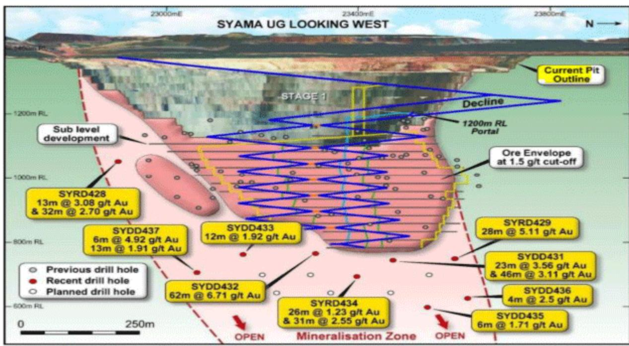
Figure 1: Longitudinal projection showing location of new diamond drill hole pierce points, results and designed underground development.
