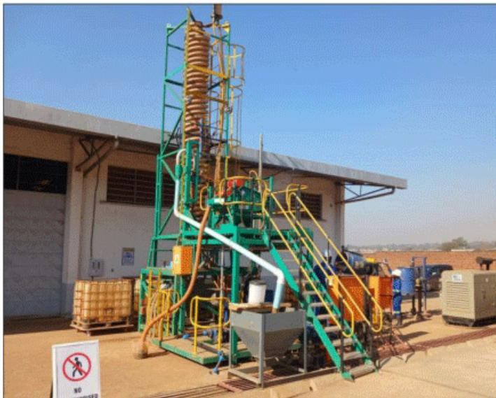
Figure 1: Installed Spiral plant at Sovereign's Lilongwe facility
