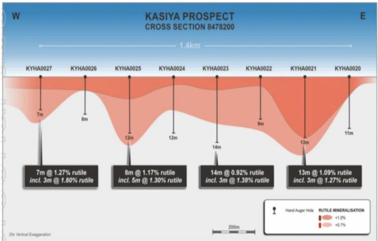
**Figure 2. Cross section 8478200 at Kasiya showing the high-grade rutile mineralisation intersected in the maiden hand-auger drilling program.**
