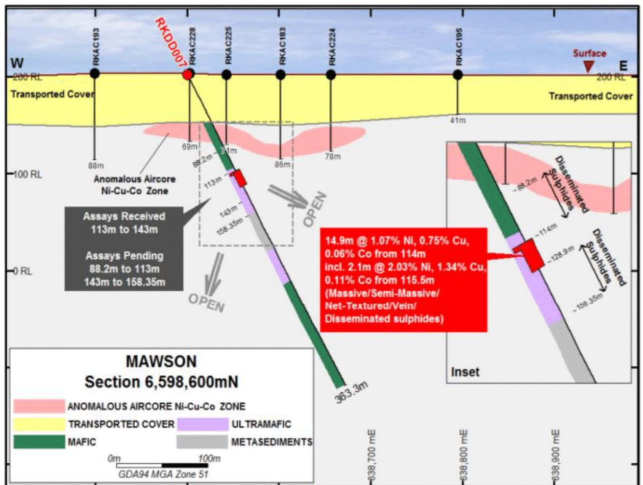
Figure 2: Drill Section 6,598,600N with Diamond Drillhole RKDD007
